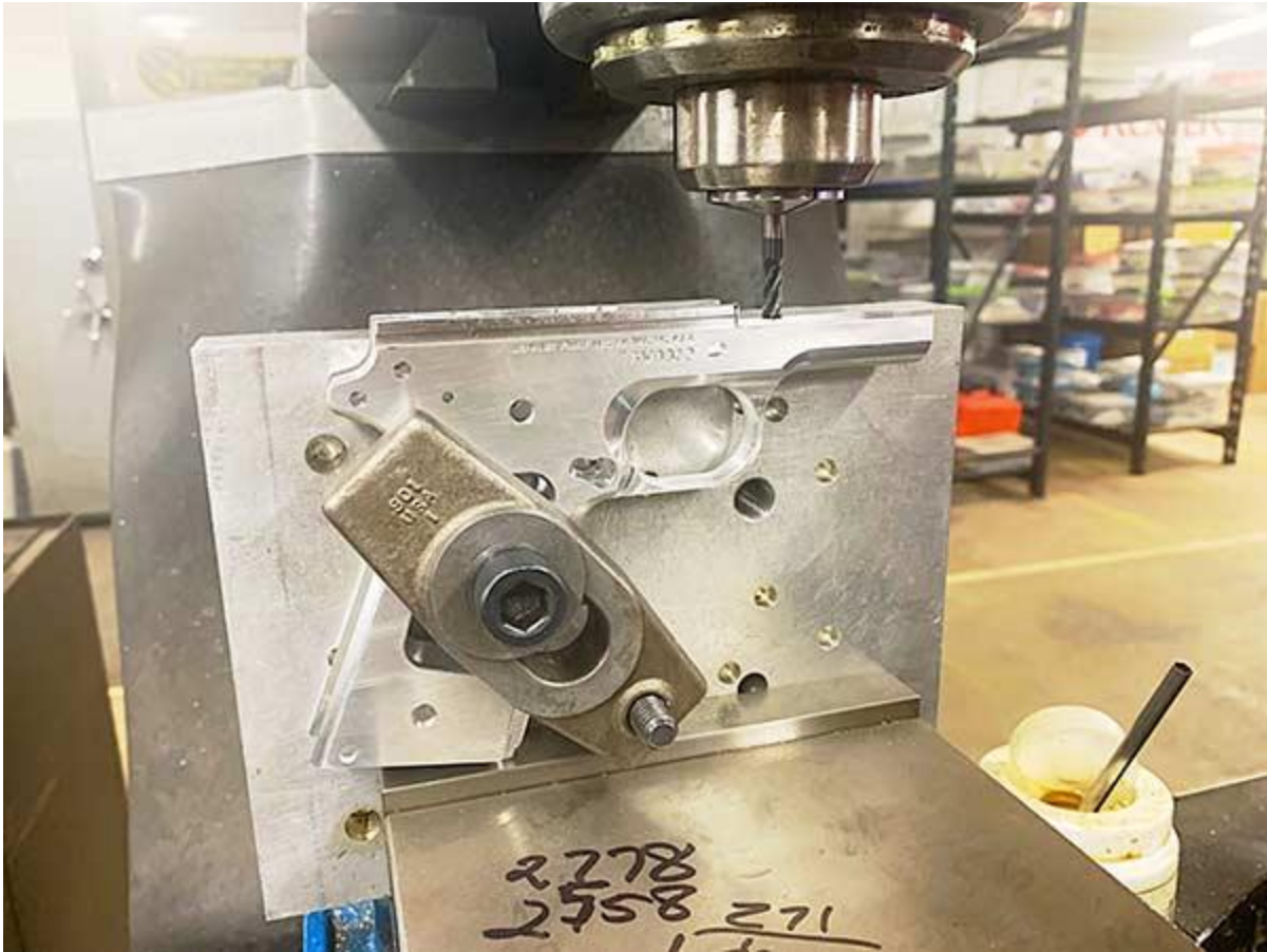
A 1911 receiver is clamped and ready to have its rails fitted for its slide.
